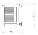
Mounting holes are 11.0mm diameter. Hole centre spacing is 155.5mm.
